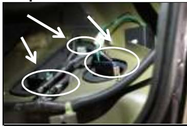
Remove the parking/brake light harness, the reverse light harness, and the turn signal light harness
