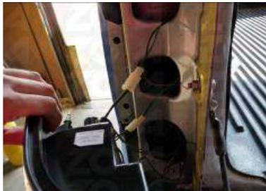
Step 7: Plug the resistors in and
