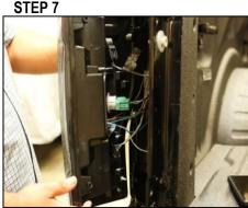
Connect factory connections to Anzo USA tail light. Slide tail light into fender well making sure guide pins go into opening.
