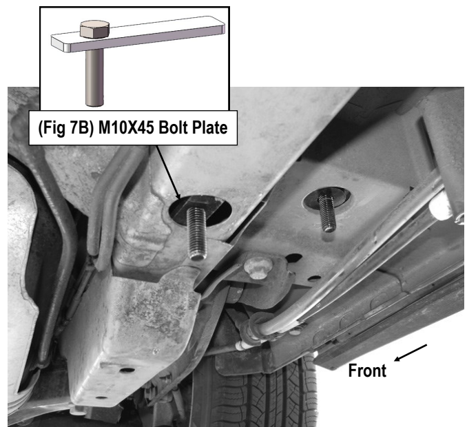
(Fig 7A) M10x45 Bolt Plate Installed (On Driver Side Rear Mounting Location)
