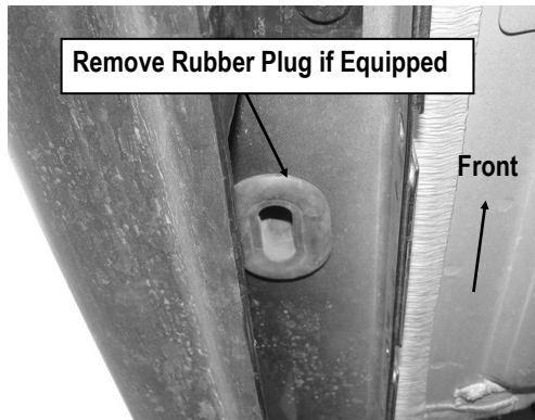
(Fig 2) Remove the Rubber Plug (At the bottom of the Rocker Panel)
