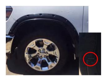
**STEP 6:** Using previously removed hex head screws, <u>loosely install</u> flare beginning at the front of the flare and working to rear. Ensure the cut-out shape fits around factory mud spat against vehicle surface. When satisfied with position, <u>completely secure</u> the (8) hex screws.
