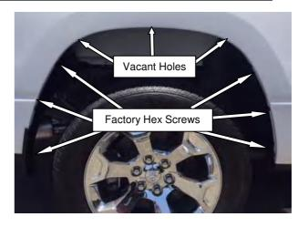
**STEP 8:** Hold Fender Flare towards vehicle in the position of best fit. Note (5) slots in Flare that correspond with factory installed hex screws, and the (3) that correspond with vacant holes in wheel arch. Remove (5) screws and retain for later re-installation.
