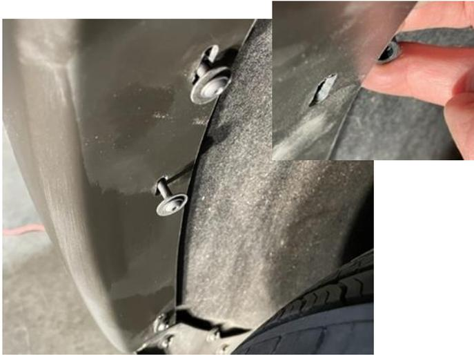
**STEP 7:** Place the smaller of the two-piece front Fender Flare on the vehicle into the position of best fit. Peel back 2" inches of the red tape liner on the fender flare rubber seal at both ends, ensure red liner can be pulled from the outside of the part. Place spacer between wheel liner and Fender Flare. Align the slotted hole in the fender flare with the hole of the spacer and begin to fasten with supplied Allen Head screw.
