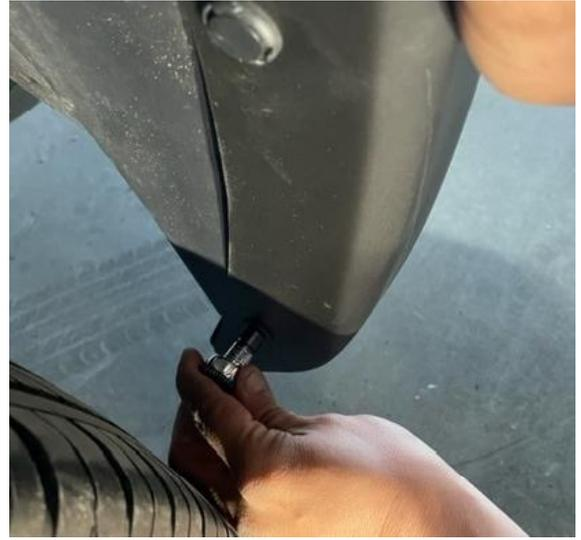
**STEP 6:** Re-install #7 Socket Head Cap Screw that was removed in STEP #4 at position "A". Repeat install steps for the opposite side.
