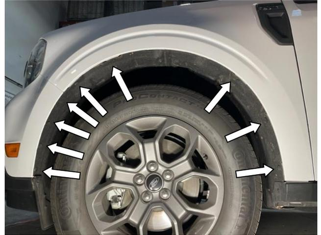
**STEP 4:** Begin by removing factory push-in plugs where noted in image above. Retain for later use in step 6.
