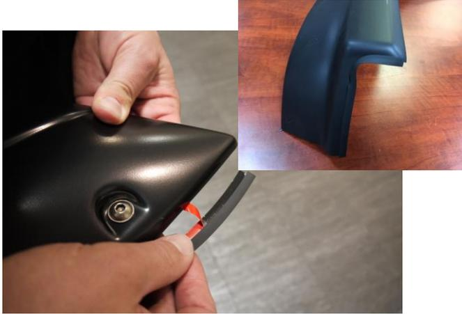
**STEP 1:** Using the supplied alcohol wipes, be sure to clean the inside of the Fender Flare where the rubber seal attaches and wipe away any residue with a dry clean cloth. Peel back 2" of the adhesive backing and position on the Fender Flare. Attach the rubber seal to the Fender Flare, peeling back the red liner a few inches at a time. Ensure pressure is used to secure rubber seal to Fender Flare edge. Attach rubber seal along all areas the Fender Flare will contact the vehicle body.
