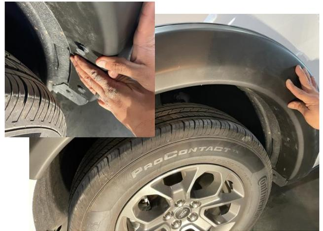
**STEP 6:** Place the larger of the two-piece front Fender Flare on the vehicle into the position of best fit. Peel back 2" inches of the red tape liner on the fender flare rubber seal at both ends, ensure red liner can be pulled from the outside of the part. Begin re-installing the factory push-in plugs at the (5) pre-existing slots in the fender flare.
