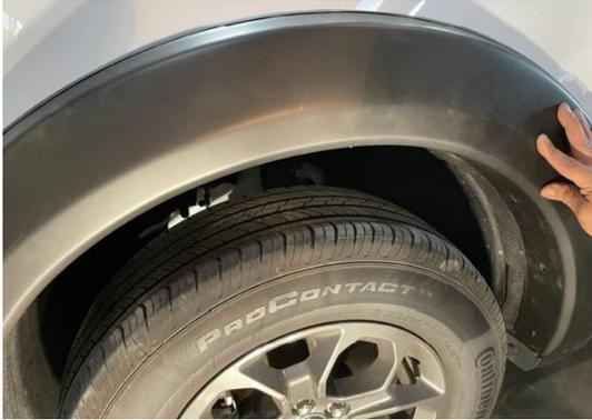
**STEP 5:** Place the Rear Fender Flare on the vehicle into the position of best fit. Begin re-installing the factory push-in plugs at the (7) pre-existing slots in the fender flare.
