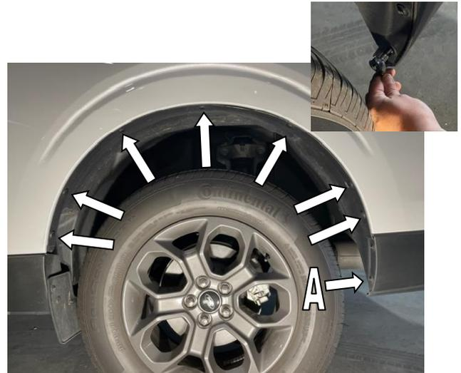
**STEP 4:** Begin by removing factory push-in plugs where noted in image above. Retain for re-install. Using #7 Hex Socket Head, remove lower screw at position "A". Retain for re-install.
