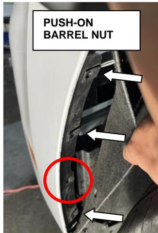
**STEP 5:** Pull the front wheel liner back enough to install the (3) push-on barrel nuts where noted in image above. Once installed, replace liner back into position and re-apply factory push-in plug in the single hole position circled above.
