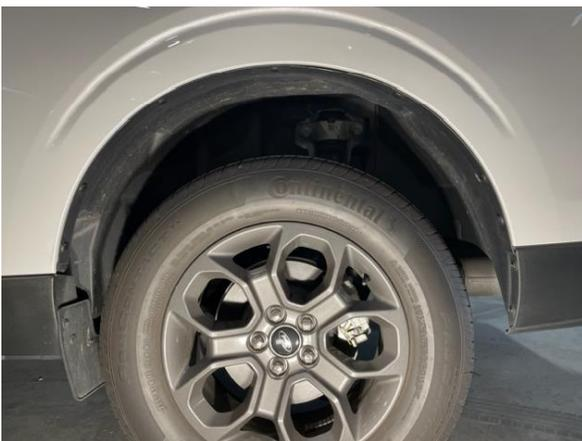
**STEP 3:** Clean the body areas where the Fender Flares will make contact. Ensure fenders are dry prior to install.
