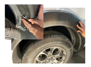
**STEP 6:** Place the Fender Flare onto the vehicle in the position of best fit. Peel back 2" inches of the red tape liner on the fender flare rubber seal at both ends, ensure red liner can be pulled from the outside of the part. Begin re-installing the factory push-in plugs at the (4) pre-existing slots in the fender flare.
