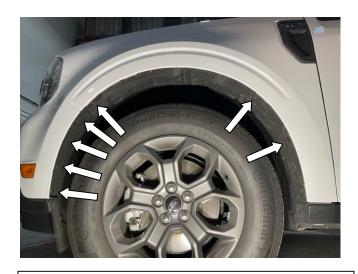
**STEP 4:** Begin by removing factory push-in plugs noted in image above. Retain for later use in step 6.
