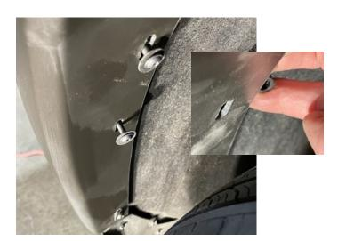
**STEP 7:** Place the provided spacer between factory wheel liner and Fender Flare. Align the slotted hole in the fender flare with the hole of the spacer and begin to fasten with supplied Allen Head screw (3). Tighten screws and be careful to not over-torque.
