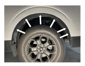
**STEP 4:** Begin by removing factory push-in plugs noted in image above. Retain for re-install at a later step.
