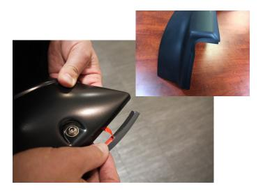
**STEP 1:** Using the supplied alcohol wipes, be sure to clean the inside of the Fender Flare where the rubber seal attaches and wipe away any residue with a dry clean cloth. Peel back 2" of the adhesive backing and position on the Fender Flare. Attach the rubber seal to the Fender Flare, peeling back the red liner a few inches at a time. Ensure pressure is used to secure rubber seal to Fender Flare edge. Attach rubber seal along all areas the Fender Flare will contact the vehicle body.
