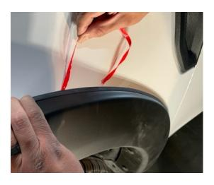
**STEP 6:** Starting at one end of the Fender Flare, carefully remove tape liner from the rubber seal a few inches at a time. Ensure rubber seal is not tucking into flare and sits flush neatly against the fender body. Apply forward pressure to adhere the rubber seal along the edge of entire length of Fender Flare once rubber seal liner is removed.
