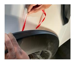
**STEP 8:** Starting at the front of the Fender Flare, carefully remove tape liner from the rubber seal a few inches at a time. Ensure rubber seal is not tucking into flare and sits flush neatly against the fender body. Apply forward pressure to adhere the rubber seal along the edge of entire length of Fender Flare once rubber seal liner is removed. Ensure all fixing points are tight and secure and that the rubber seal is flush and properly seated against the vehicle body.
