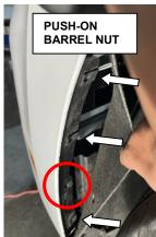
**STEP 5:** Pull the front wheel liner back enough to install the (3) push-on barrel nuts noted in image above. Once installed, replace liner back into position and reapply factory push-in plug in the single hole position circled above.
