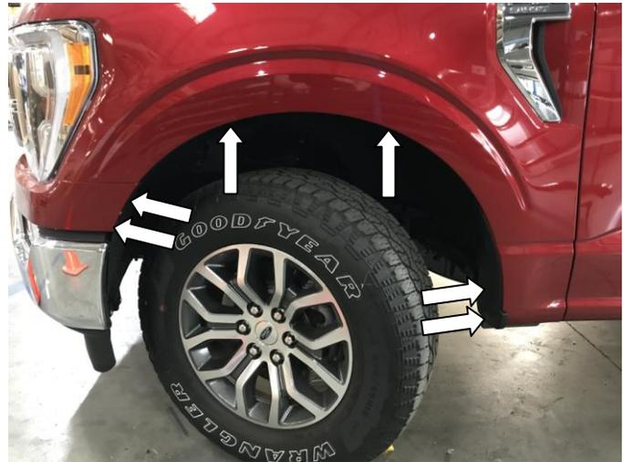
**STEP 6:** Locate six 7mm bolts in the vehicle wheel well.
