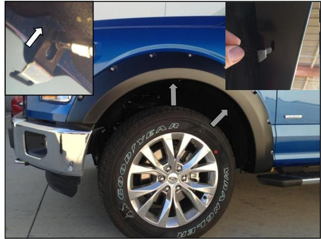
**STEP 8:** Place the Fender Flare onto the vehicle and fit into the correct position following the contours of the body. Use 2 of the retaining clips and 7.0mm bolts to secure the Fender Flare to the body. Make sure the clip securely engages the Fender Flare.
