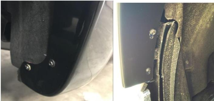
**STEP 9:** Reinstall the remaining 7mm bolts, two at the front bottom corner and two at the rear bottom corner.
