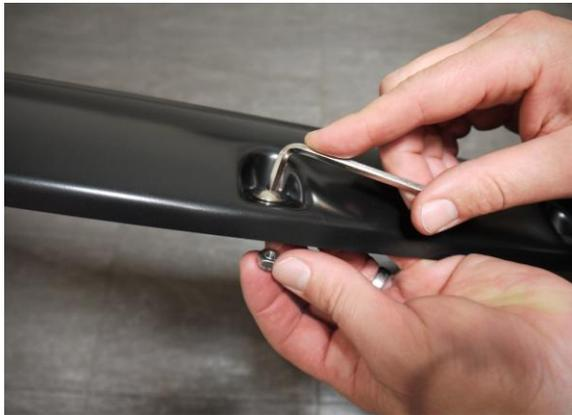
**STEP 1:** Attach the bolts and nuts to each Fender Flares using a 3/16" Allen key and a 10mm wrench/socket (wrench /socket and Allen key not supplied). Ensure inside of Fender Flares where the rubber seal is attached is clean, using the alcohol wipes provided. Wipe away any residue with a dry clean cloth.
