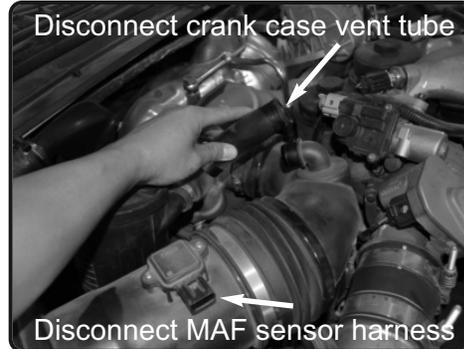
3. Disconnect the crank case vent tube from the factory air duct and MAF sensor harness from the MAF sensor on the air box assembly.
