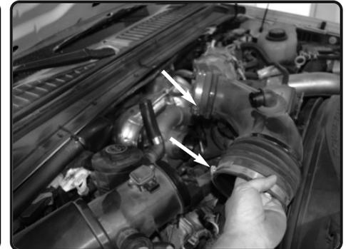
4. Loosen the two clamps on the factory air duct and then remove the entire factory air duct.
