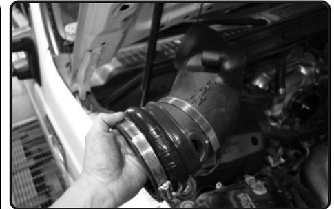
**16.** Place the 4.50" hump hose and two #72 clamps onto the big end of the Injen intake tube. You will have to slip the entire hump hose over the tube to make room to install the tube onto the Injen air box.
