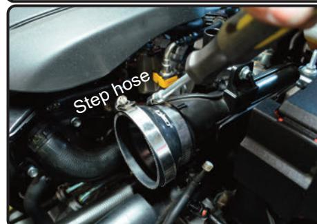
11. Secure and tighten the clamp on the turbo housing only using 8mm nut driver.
