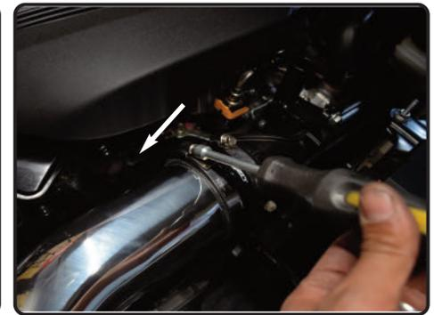
**16.** Adjust and tighten the clamp on the intake tube using 8mm nut driver.
