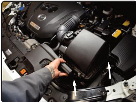
6. Carefully lift up the air box assembly.
