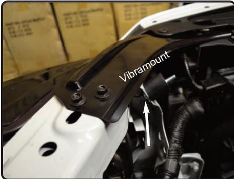
**13.** Secure the backside of the vibramount using provided M6 nut and fender washer.
