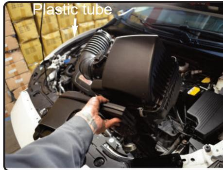
7. Remove the air box assembly out of the vehicle.
