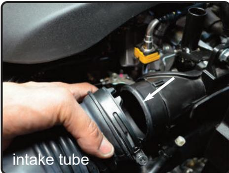
5. Pull back the intake tube away from the turbo housing.
