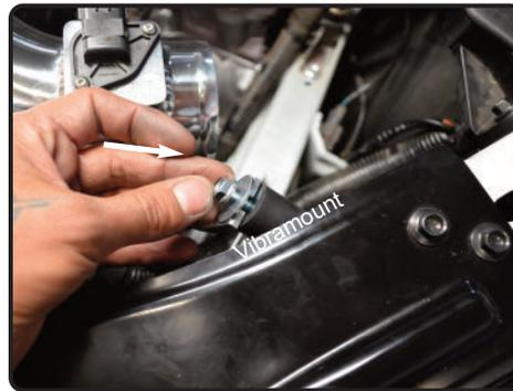
**14.** Attach the provided M6 nut and fender washer to the top of the vibramount. Do not tighten.
