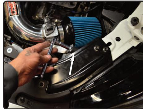
**19.** Adjust the intake for fitment and tighten the bracket using 10mm socket or wrench.
