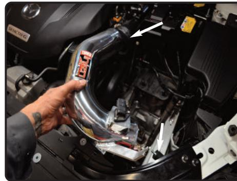
**15.** Install the intake tube and position to the step hose and bracket to the vibramount.
