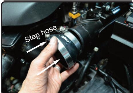
10. Install the provided step hose with clamps provided to the turbo housing.
