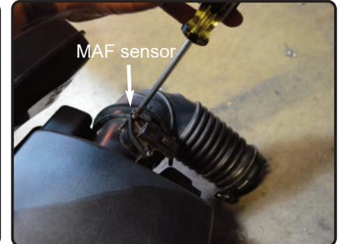
8. Remove the 2 screws holding in the MAF sensor.
