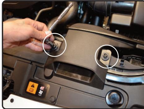
2. Remove the 2 screws holding in the top of the factory ram scoop. Remove the 2 screws using 10mm socket or wrench.
